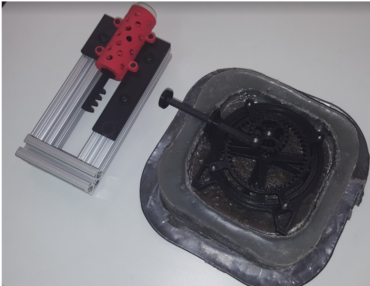
Figure 3-5: An example of a composite part manufactured by combining a regolith analog with a polymer binder. The resulting structure exhibits excellent tensile and compressive properties, and can be bonded with a fully polymer part (shown inserted as a gear and piston assembly manufactured from ABS plastic)
