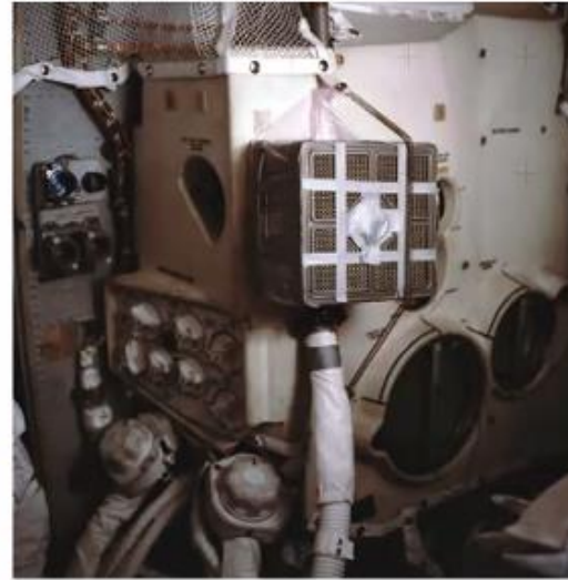
Apollo 13 crew improvised to adapt the CM's lithium hydroxide canisters for use in the LM (NASA). Skylab 4 astronauts Gerald P. Carr, left, and Edward G. Gibson trimming their homemade Christmas tree
